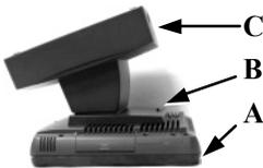
**Step B:** Press the Lock/Release button for main unit detach and meantime ...
