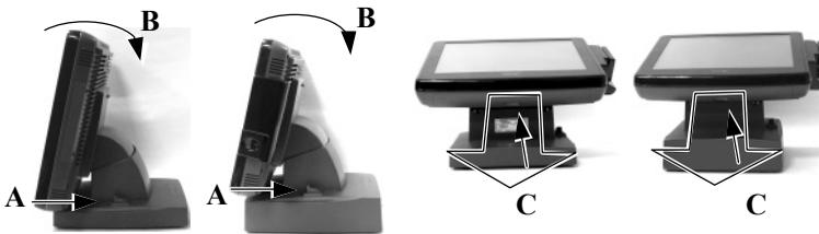
**Step A:** Push lock/release lever for tilt angle adjust backward
