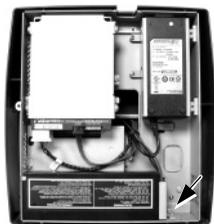
Please remove the UPS battery bracket fixing screw and slide right the UPS battery bracket to take it out for universal base model as in left picture. Put the battery in at the other end first and remount the bracket with its tongue matching under a bridge in the wall of base box from the right as arrowed in above left picture then apply the fixing screw. Please
