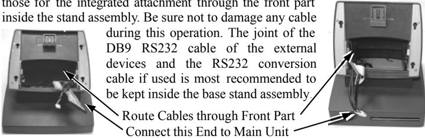
Now, turn the adjustable stand assembly back to normal orientation and arrange all cables to come out of the area for mounting main unit from the bottom edge for ease of later operation.
