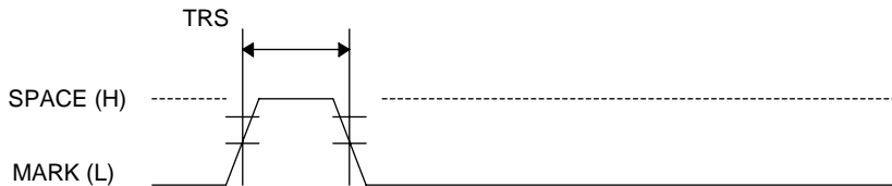
Figure 2.1.2 Minimum Reset Pulse Width (pin 25)
