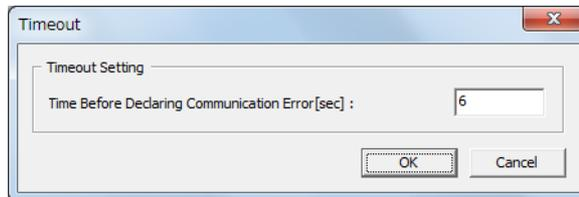
In this window, you can set the timeout time for communicating with a network interface. A communication error occurs if this time is exceeded.
