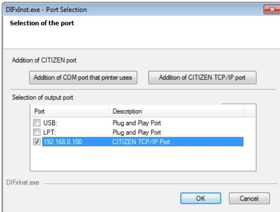
\* If status function is used through standard TCP/IP port, there could be trouble of PC freeze by waiting for status data from printer.
