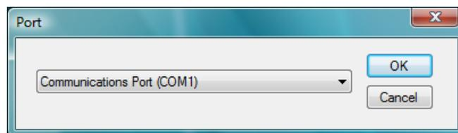
Set the details of port for serial communication condition accordingly and press "OK".
