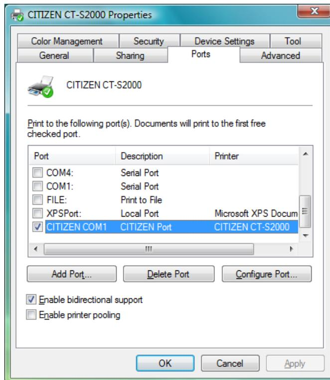
\* If status function is used through normal serial port without choosing CITIZEN COM, there could be trouble of PC freeze by waiting for status data from printer for about 30 seconds.
