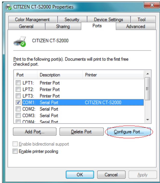
Please change the setting according to the serial port condition of printer and press "Apply".
